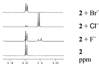
**Figure 2.** The amide NH region of overlaid  $^1\text{H}$  NMR spectra of free **2** and the 1:1 mixture of **2** with  $(n\text{-Bu})_4\text{NF}$ ,  $\text{Ph}_4\text{PCl}$ , and  $\text{Ph}_4\text{PBr}$ , respectively (3 mM in  $\text{CDCl}_3$  at  $-30^\circ\text{C}$ ).
